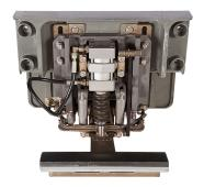
Current collector devices are used by Metro to collect the energy from the third rail to energize the Electrical Multiple Unit installed in the trailers.
