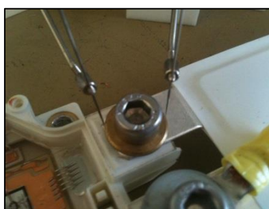
Figure 8. Resistance across the contact area measurement—module M.
