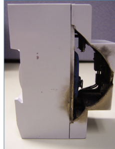
Figure 3: TVSS damage due to abnormal overvoltage test.
