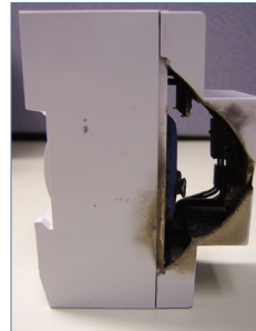
Figure 3: TVSS damage due to abnormal overvoltage test.
